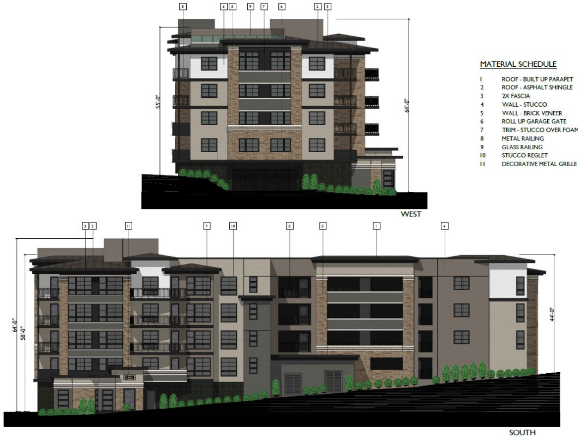
Figure 3a. Building Elevations (West and South)
